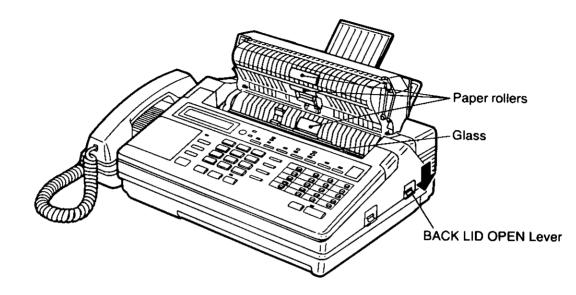
If you cannot get a clear copy after performing the above steps 1 and 2, clean the thermal head with a cloth moistened with denatured alcohol (alcohol without water), then dry thoroughly. To prevent malfunction due to static electricity, do not use a dry cloth and do not touch the thermal head with your finger directly.
